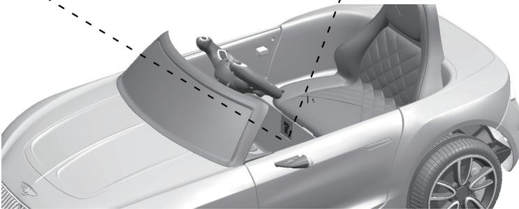
1. Plug the charger port into the input socket. (the socket is below the seat)
