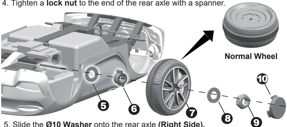
5. Slide the **Ø10 Washer** onto the rear axle (**Right Side**).
