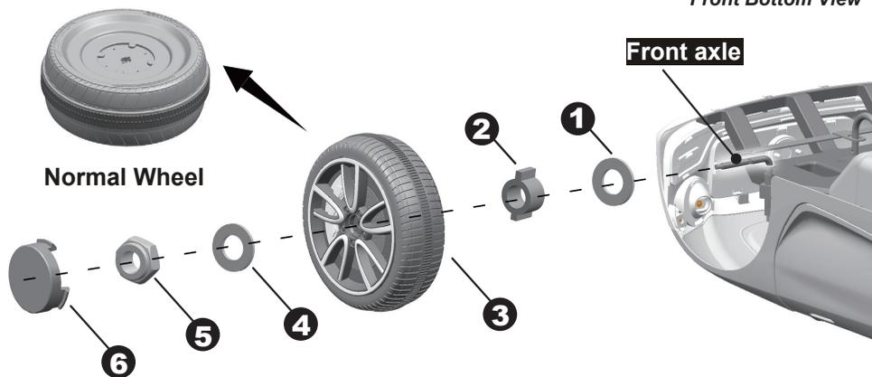
Remove all the parts from the front axle.
