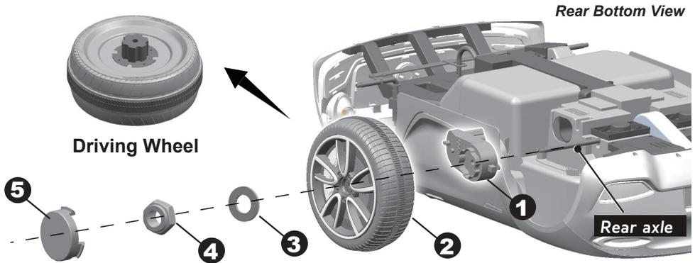
1. Slide the **gear box** onto the rear axle. “R” labeled gear box should be fit to the “R” side of vehicle body; “L” labeled gear box should be fit to “L” side of vehicle body. Keep the motor and the connector on the gear box pass through the larger hole on the rear of the vehicle and out where the battery sits.
