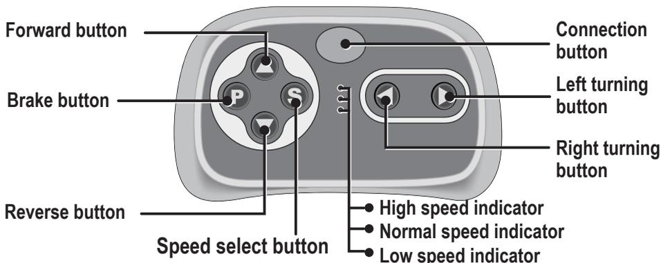
The remote control has precedence over foot pedal operation.
