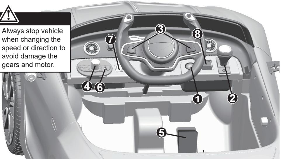
1. **Power Switch:** Turns the vehicle on and off.
