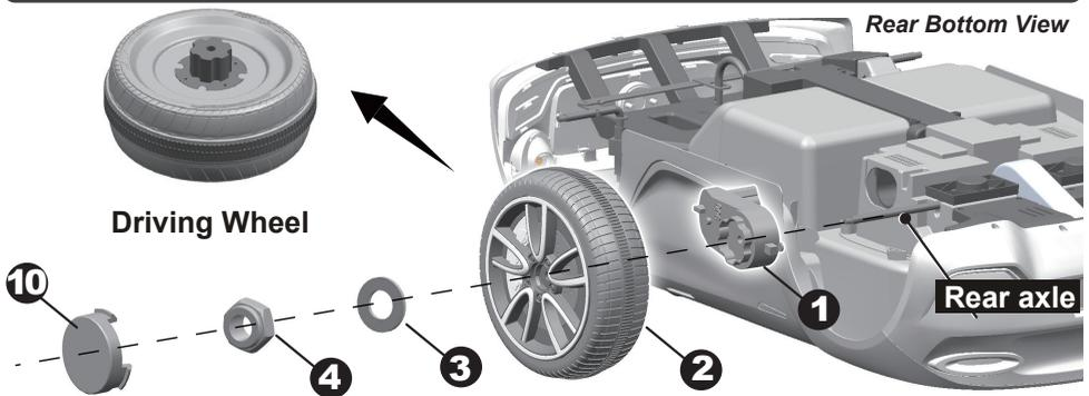
1. Slide the **gear box** onto the rear axle (**Left Side**). Keep the motor and the connector on the gear box through the larger hole on the rear of the vehicle and out where the battery sits.
